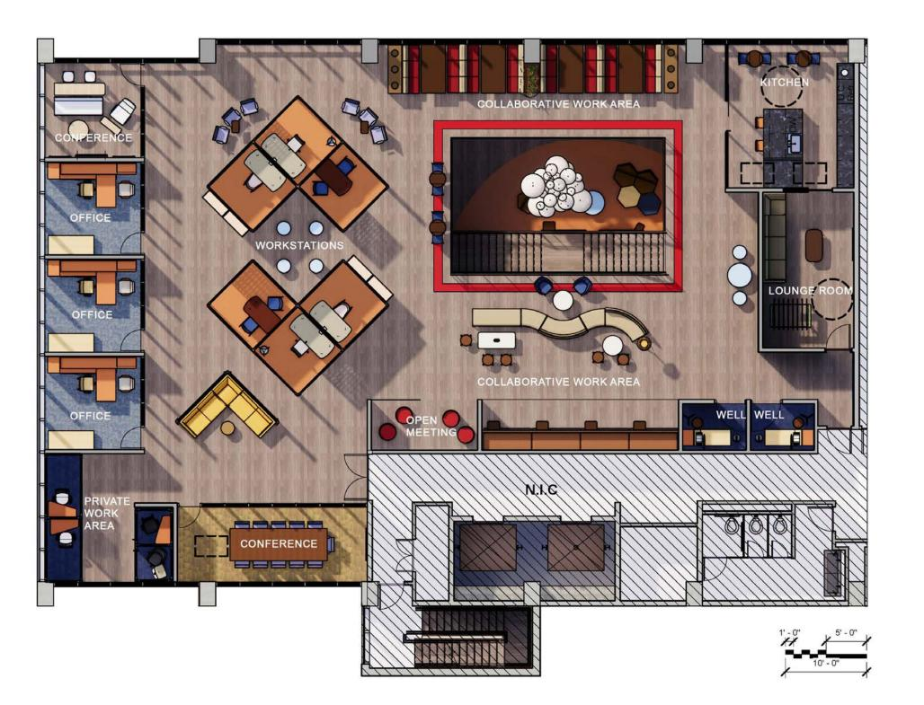
The second floor houses the breakroom and work area for those higher in the chain of command. The design utilizes a variety of ceiling types and heights to define zones and for wayfinding.
